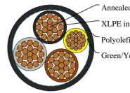
Annealed copper conductor XLPE insulation Polyolefin outer sheath Green/Yellow wire
